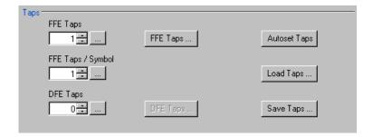
Pressing the FFE Taps... button displays a dialog showing the current FFE tap values. You can specify each FFE tap coefficient individually. Pressing the Defaults button sets the first FFE tap to 1 and the rest to 0.
